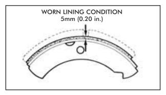
Shoe tips should be inspected and cleaned at this time. If the flat length exceeds 28mm (1.10 in.), the shoes should be replaced.
