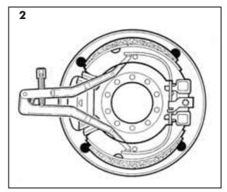
The Meritor Spring Expander Tool (Fig. 1) is designed to permit the removal of the brake shoes from the F.C.S.S.A (S.A.C) type brake without the need to remove the brake hub or disturb the in-axle setting of the A.B.S. sensing mechanism.
